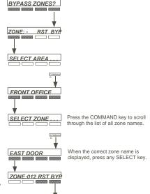
The display shows the zone number. Press the SELECT key under **RST** to Reset the zone. Press the SELECT key under **BYP** to Bypass the zone.
